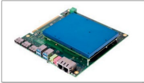
Figure 4. The carrier board MB-COME6-3 is designed for COM Express Type 6 modules and offers PCIe x4 and PCIe x16 high bandwidth connectivity to add-on cards which are used in high-performance AI solutions, for example.
