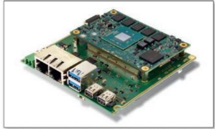
Figure 2. A modular approach enables scalability and flexibility. The TQ standard carrier board MB-M10-1 in combination with COM Express Mini modules like Intel Atom based TQMx38M builds the heart of very compact, robust and powerful IoT applications.
